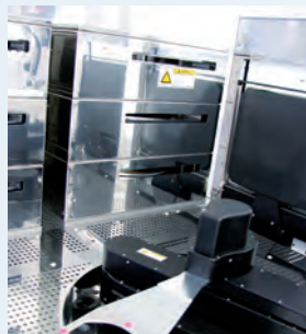
EVG ® 150 300 mm stack of Bake, Chill and Vapor Prime Modules
