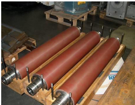
Incoming wire guide rolls for Diamond wire or slurry using machines
