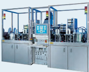
HERCULES® Lithography Track System with coat/expose/develop configuration
