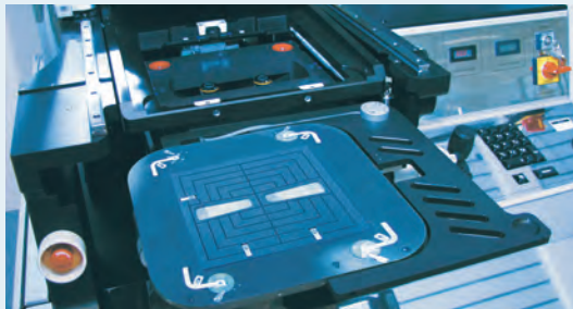
EVG®6200 ® With proximity wafer chuck for square substrates
