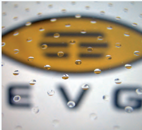
Microlens structures for WLO modules fabricated utilizing UV-NIL
