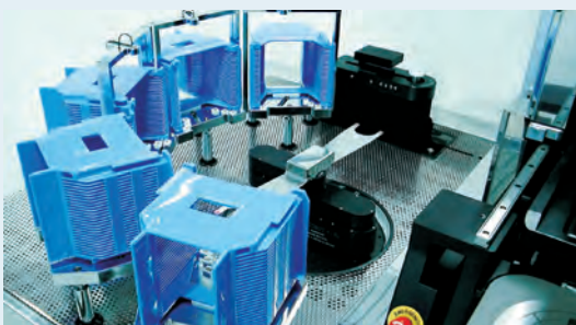
EVG®620 Wafer Handling Module with 5 cassette stations
