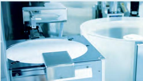
IR-inspection station for pre-bonding on EVG®301
