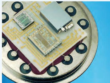
MEMS capacitive accelerometer **Courtesy of Colibrys**
