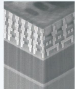
Cross-section of CMOS SOI Wafer after double bonding/ thinning, BCB ashing and sawing **Courtesy of Freescale**
