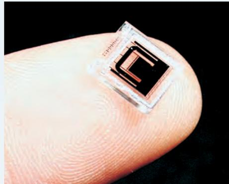
Flow sensor chip, MEMS chip made utilizing wafer bonding **Courtesy of ISSYS**
