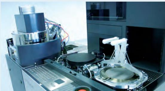
Cooling station and handling tool on EVG®520IS
