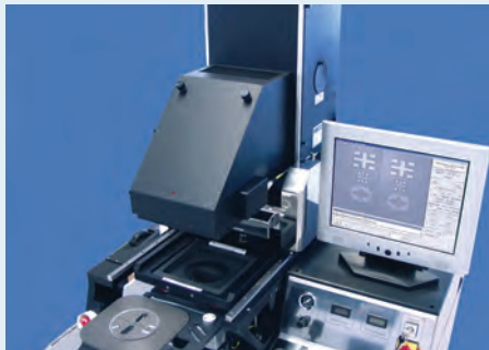
EVG®620 Mask aligner for single step UV imprinting
