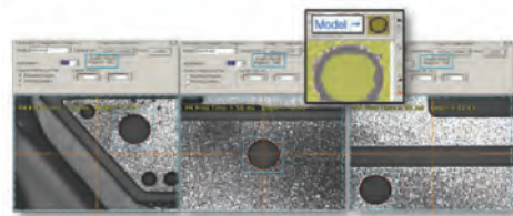
Robust PR (GS4) with Feature Find and Geometric Model modes developed for difficult patterns like direct bonded copper (DBC) substrates
