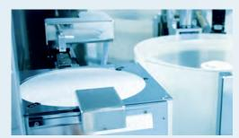
IR-inspection station for pre-bonding on EVG®301
